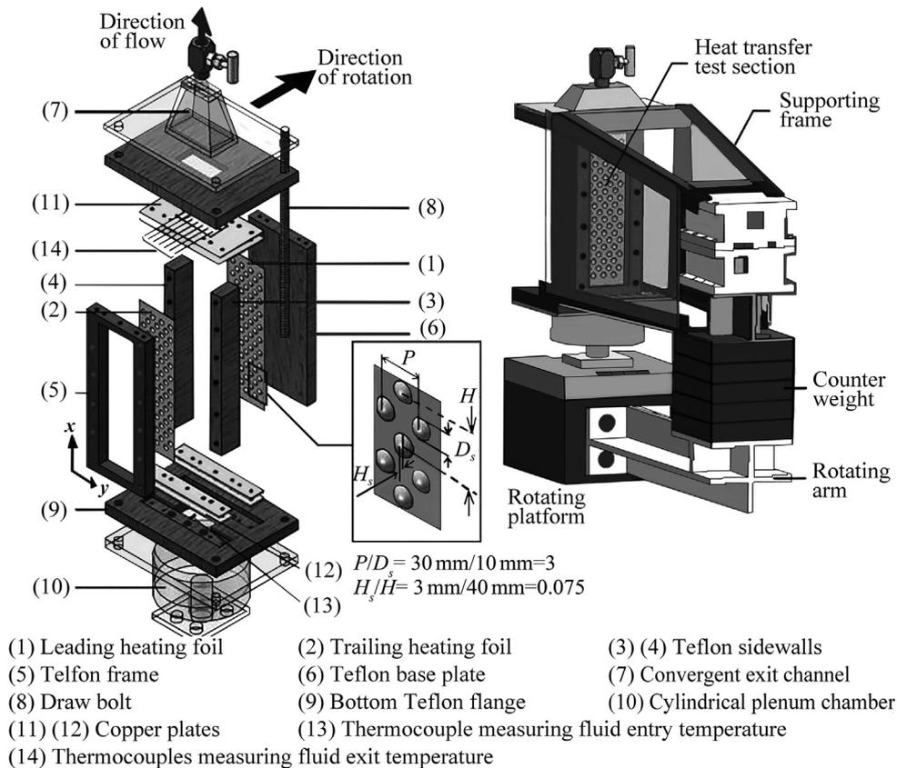
**Figure 5** Schematics of the measurement setup using infrared thermometry by Liou and colleagues [38,39].
