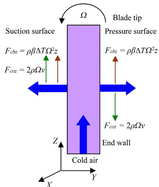
**Figure 9** The action of Coriolis force and centrifugal buoyancy force on a rotating blade, from Tao et al. [57].
