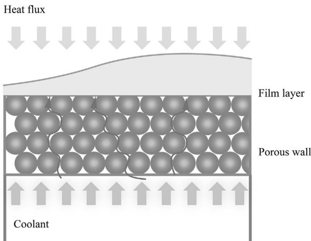
**Figure 13** Schematic of effusion cooling structures studied by Jiang et al. [129].
