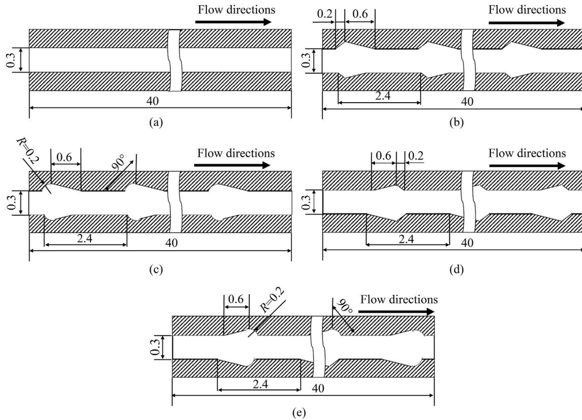
**Figure 12** Schematic diagram of crater structures studied by Huang et al. [123]. (a) Straight channel; (b) triangle A; (c) a combination of 90° fan and triangle; (d) triangle B; (e) a combination of triangle and 90° fan (unit: mm).
