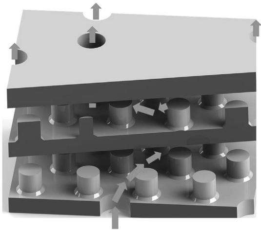
**Figure 10** Schematic diagram of lamellar cooling structure, Bunker [115].
