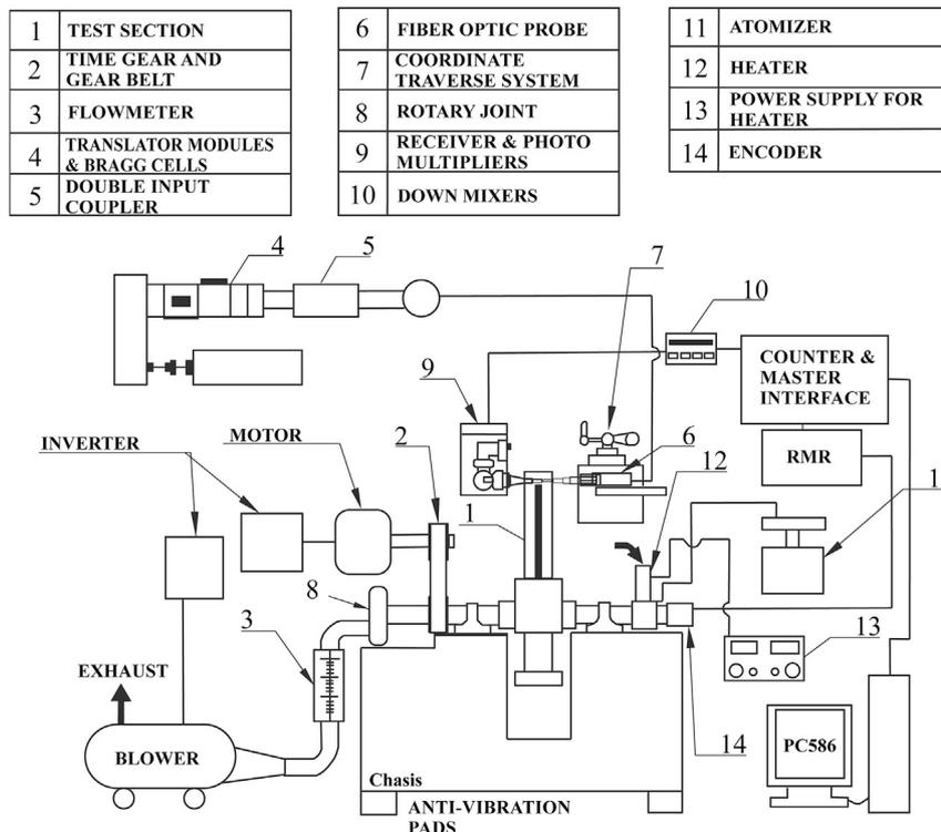
**Figure 3** Rotating LDV equipment adapted by Liou and colleagues [39].
