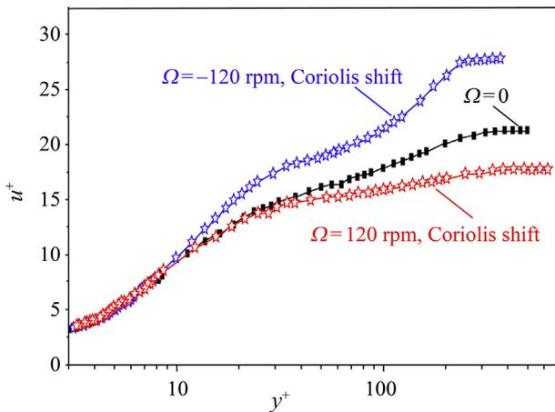
Figure 7 Velocity distribution in iso-thermal boundary layer under rotating conditions (Tao et al. [15]).
