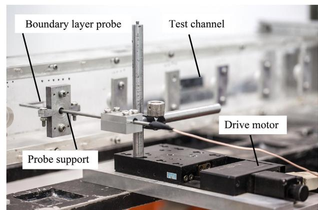
**Figure 1** Rotary hot wire equipment adapted by Tao and colleagues [15–17].
