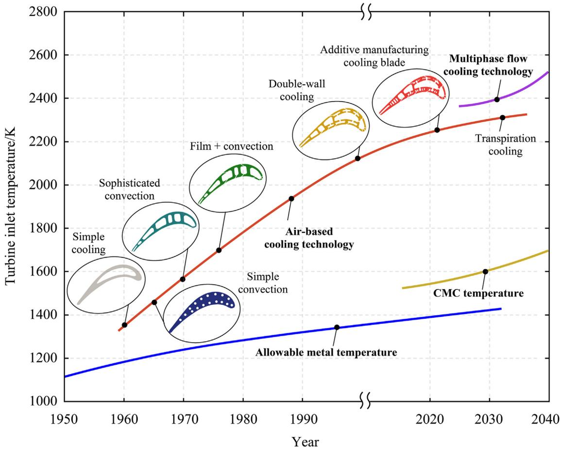
Figure 6 Evolution of turbine blade cooling technology (extended from Clifford [43]).
