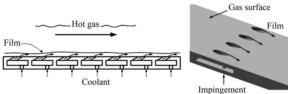
**Figure 11** Schematic diagram of double-wall cooling, Wang et al. [120].
